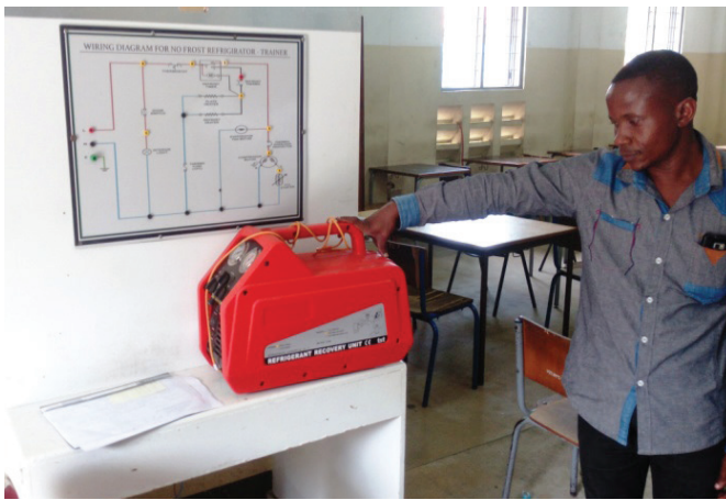
Saidi Mziwanda shows a refrigerant recovery unit and a recovery cylinder at VETA Chang'ombe, Dar es Salaam
