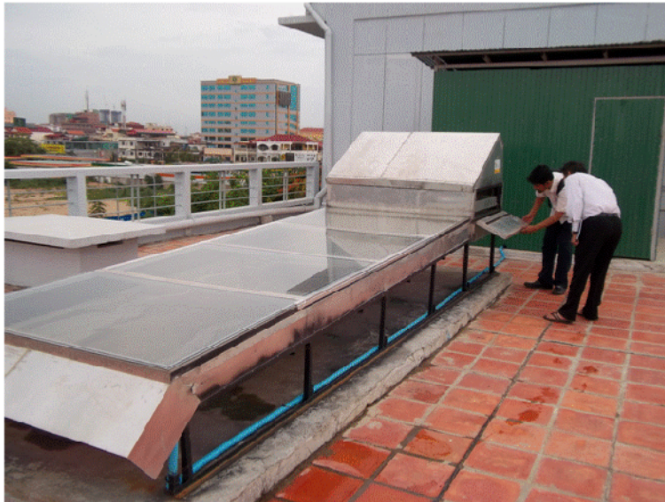
Figure 1.5 The experimental natural convective solar dryer located on roof top
