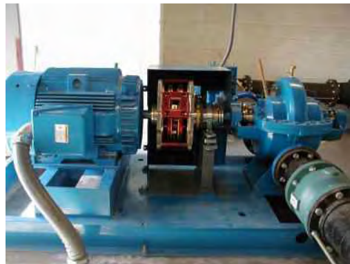
Fig. 9.16. PWM and magnetic variable speed drives (courtesy of Robicon and MagnaDrive)
