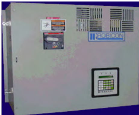
Fig. 9.16. PWM and magnetic variable speed drives (courtesy of Robicon and MagnaDrive)
