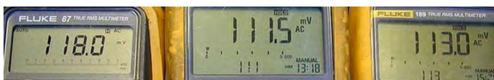
Fig. 12.29. Amp Measurements for Each Phase
