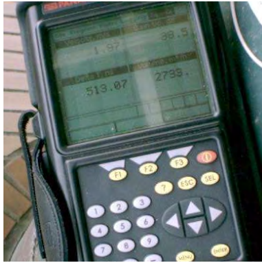
Fig. 12.22. Transit-time ultrasonic flow meter
