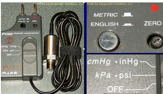
Fig. 12.14. Inaccurate Pressure Gauge and PV-350 Pressure Indicator
