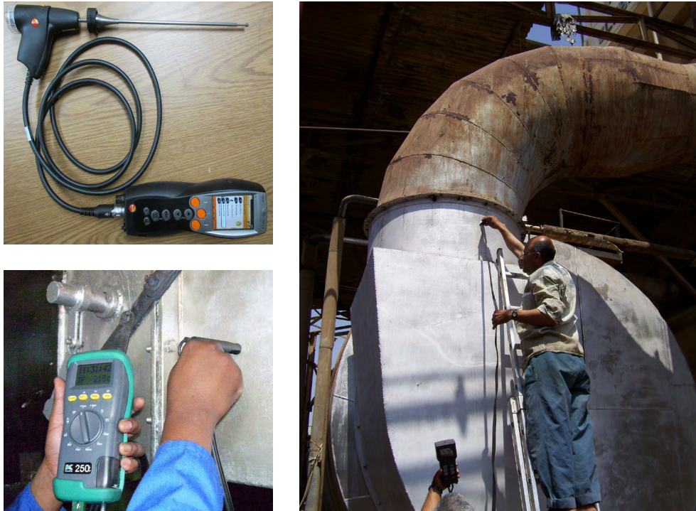
Figure 40: Use of Stack Gas Analyzers in a Steam System Assessment
