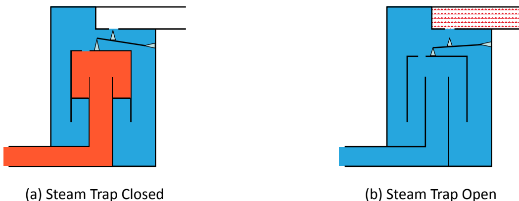
Figure 26: Functioning of Inverted Bucket Mechanical Steam Trap (Courtesy: US DOE Steam BestPractices End User Training)
