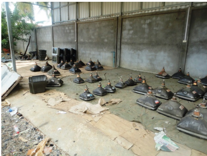
Figure 2. Televisions (CRT) dismantling and reassembling in Banteay Meanchey (personal picture).
