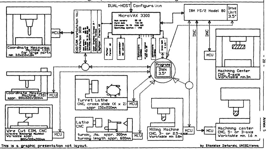
The computer hardware and peripheral equipment for PHASE 1 of the pilot CAD/CAM project.
