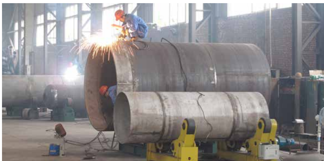
Workers in Sichuan Guoli Energy Science & Technology Co. Ltd are making new boilers used to recover waste heat.
