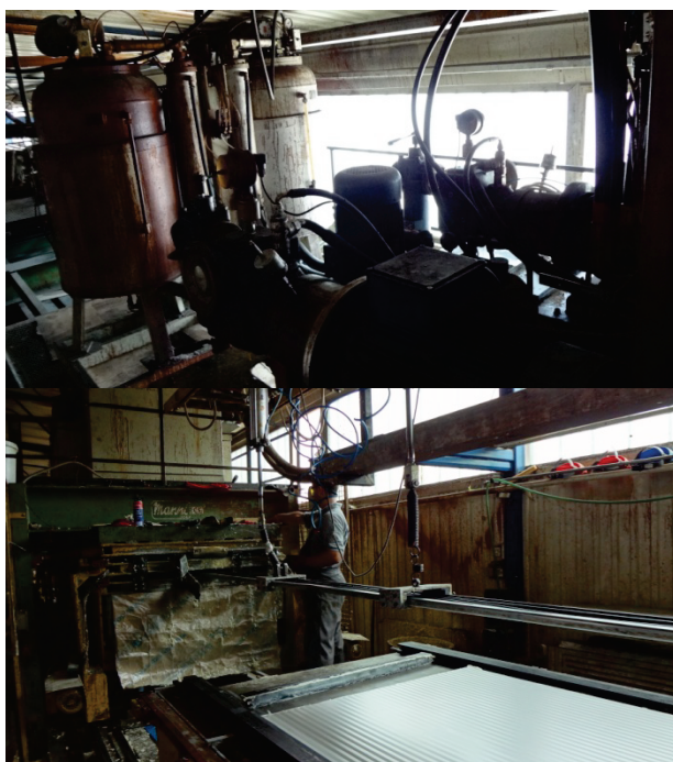
Illustration 2.: SAIP foaming machine and preparation before injection.
