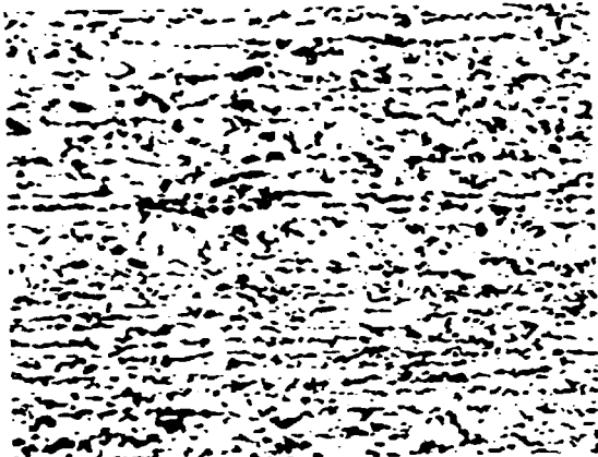
Photomicrograph 5. Magnification: 100X; Etchant: 3% Nital. Microstructure of the base metal (similar structure for all 3 heats) showing polygonal grains of ferrite and pearlite. The ASTM grain size is finer than ASTM No. 8
