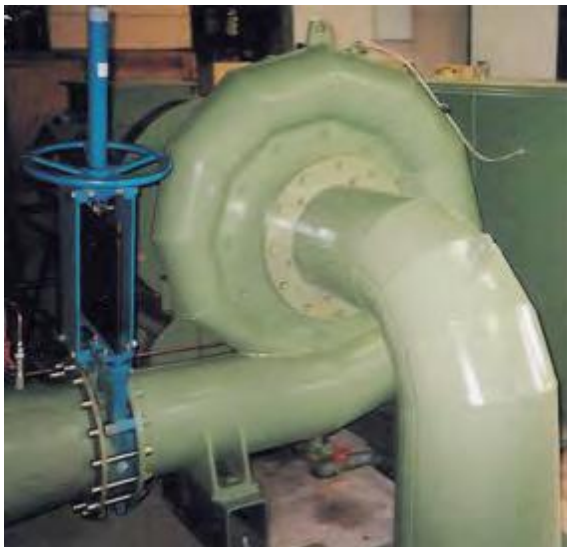
Figure 13: Horizontal Francis Turbine
