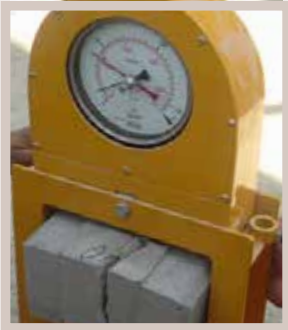
COMPRESSIVE STRENGTH TESTING OF HYDRAFORM BLOCK
