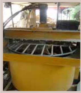
Ribbon pan mixer for preparation of composition for moulding blocks
