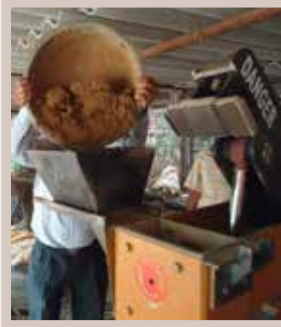
The hopper is filled with raw material before moulding
