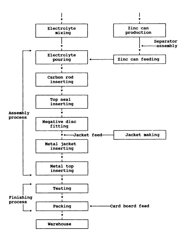
FLOW CHART ALKALINE DRY CELL BATTERIES PLANT
