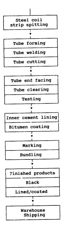
FLOW CHART WELDED STEEL PIPES PLANT
