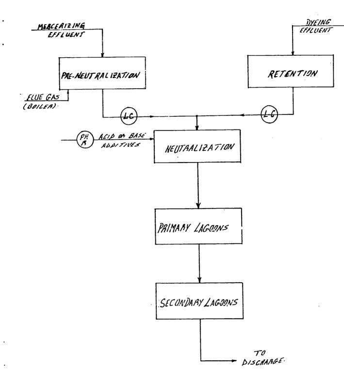
The factory has a treatment plant which is built at the cost of Birr 1,865,506.04. The plant is mainly composed of a neutralization plant and aerating lagoons.
