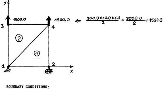
NODE 1,  $U_{4}=0$ ,  $V_{4}=0$ NODE 2,  $V_{2}=0$  A6 - 5
