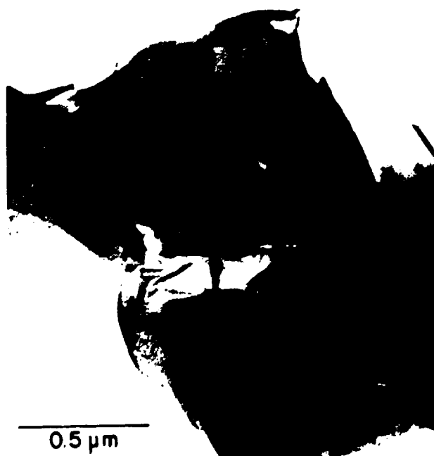
Fig. 3.36. Wyoming-type montmorillonite aggregates in the top layer Parys bentonite (sample 51) from South Africa.
