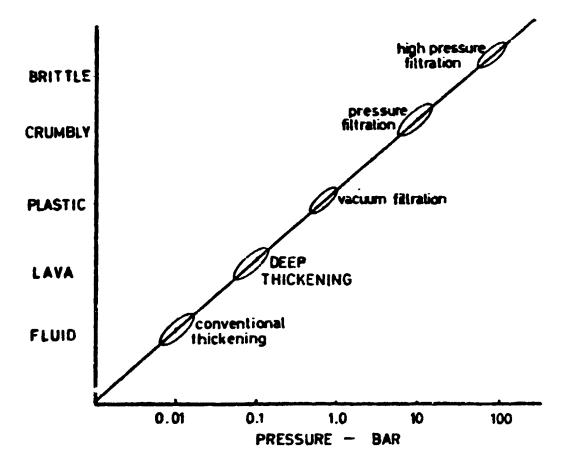
FIG. 2: How Pressure used in separation affects physical properties of red mud.
