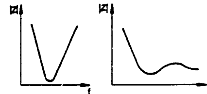
Fig. 22. Absorption circuit of one harmonic and high pass filter of higher harmonics and their impedance curves.
