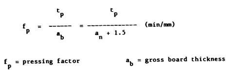
t = pressing time a = net board thickness n When the operation time is longer (in difficult working conditions during
