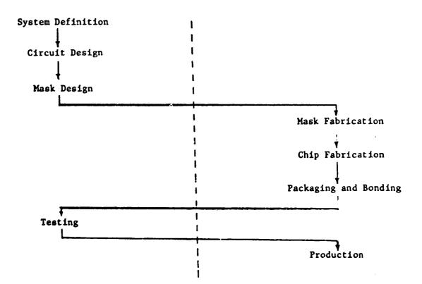
The silicon foundry approach to integrated circuit design is aimed at completely restructuring the semiconductor industry in such a way that anyone with an idea can get that idea cast in silicon at a reasonable cost. To achieve this end the "thought stages" associated with design are separated from the "mechanical stages" associated with fabrication (see figure I).
