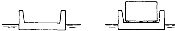
Loose sectional dock
