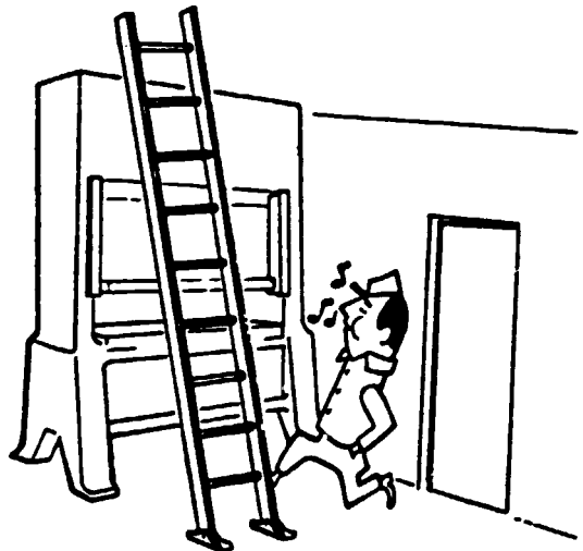
Use caution when placing a ladder near aisles or doorway - install warning signs and barricades.
