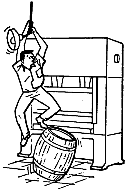
Never use barrels, boxes, crates, stools, or similar items as substitutes for scaffolding.
