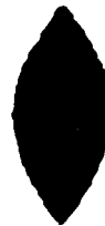
(c) The reason for the pattern spreading in the middle could be: too narrow a spray; too low a pressure or paint is too thick; too small an air cap with pressure feed; or too large a spray head.
