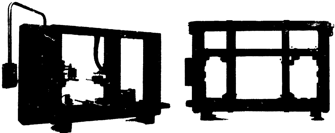
Figure 175. Pneumatic carcass clamps with cylinders (left) and with fire-hose pressure units (right)
