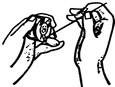
(a) Cleaning side openings
