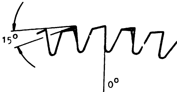
F. Front bevel angle = 15° Back level angle = 15°
