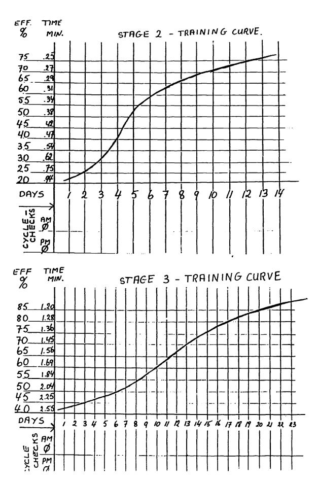
The progress of the operator against the training-curve is obtained by taking the average of 5 cycle times of the operation (use a stopwatch with 1/100 of a minute values). The operator can be checked many times per day but it is normal practice to make an entry on the graph once in the morning and once in the afternoon.
