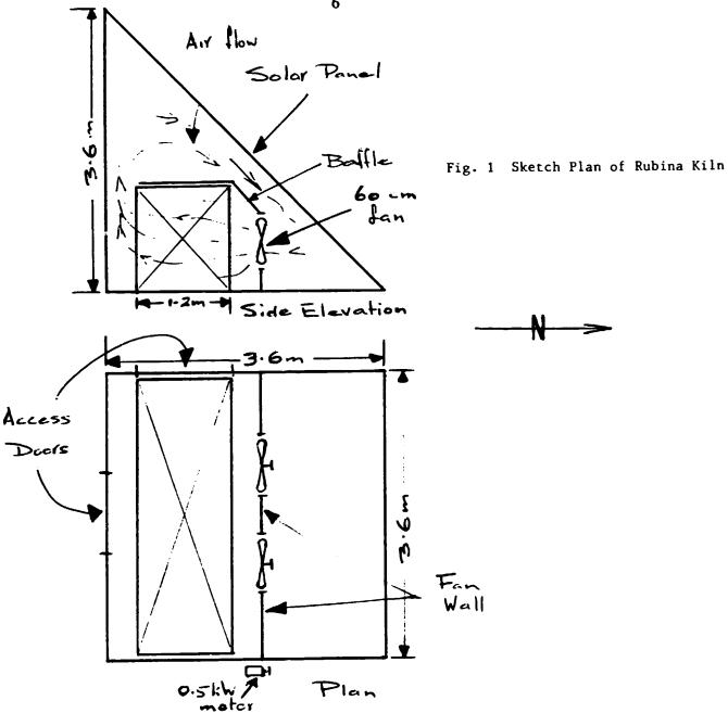
The solar panel is of corrugated, fibreglass reinforced polyester and the floor, east, south and west walls are of plywood sheet and timber frame construction, with polystyrene foam insulation in the cavity. The two, 60 cm, non-reversing fans are driven by a single 1.5 kW motor.
