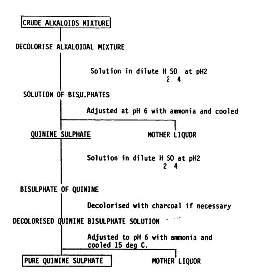
Alkaloidal materials recovered by alkaline treatment of the mother liquors to be processed separately for production of quinidine and other cinchona alkaloids.
