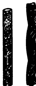
Figure 5. Left, spirally wound tube which, according to theory, buckles under axial tensile strain to the form indicated on right (lit. 5).
