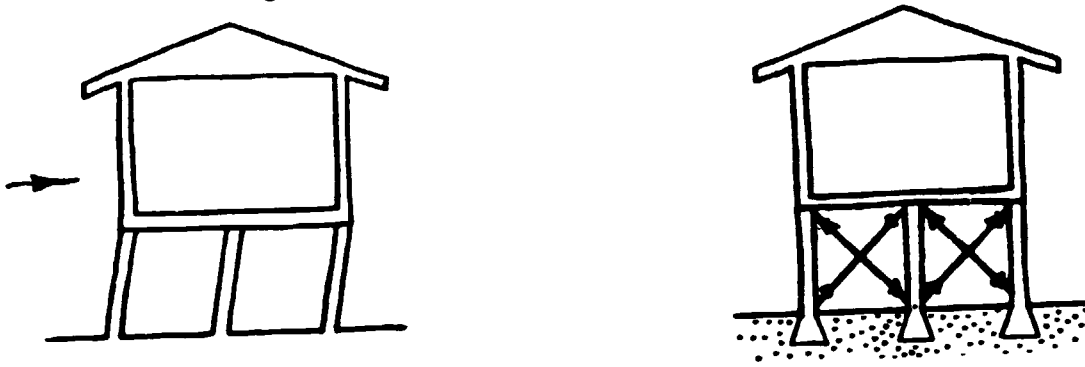
Figure 14 - Bracing of the sub-floor support system
