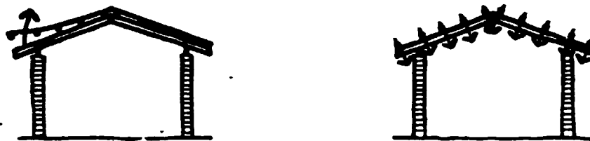
Figure 3 - Battens lifting from rafters due to the failure of batten fasteners
