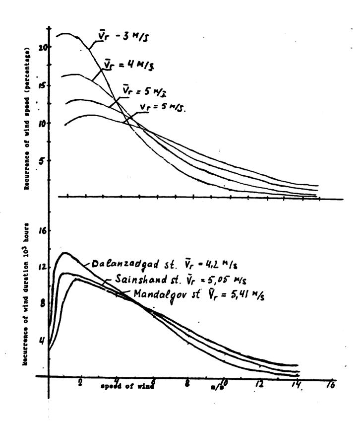
Figure II. Wind speed of wind stations, including speed at the station for desert and semi-desert zones of Mongolia
