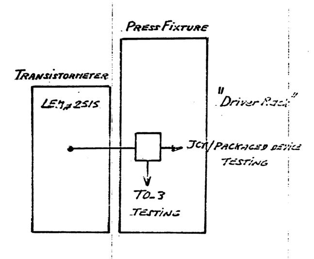
Fig. Transistormeter / Press fixture Connection
