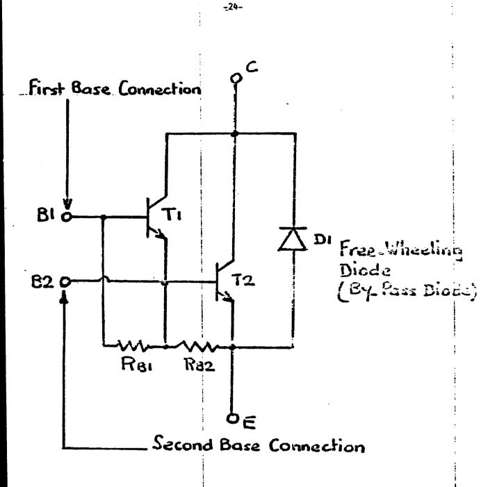
Fig 2. Darlington Transistor Schematic
