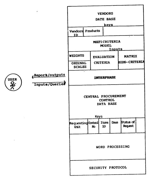
Figure 2. Basic structure of Proposed System
