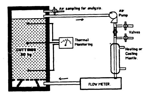
Figure 3. Proposed laboratory apparatus designed to eliminate moisture- and temperature gradients from piled jute cuttings and maintain an optimum temperature (65°C) for pectinase activity.
