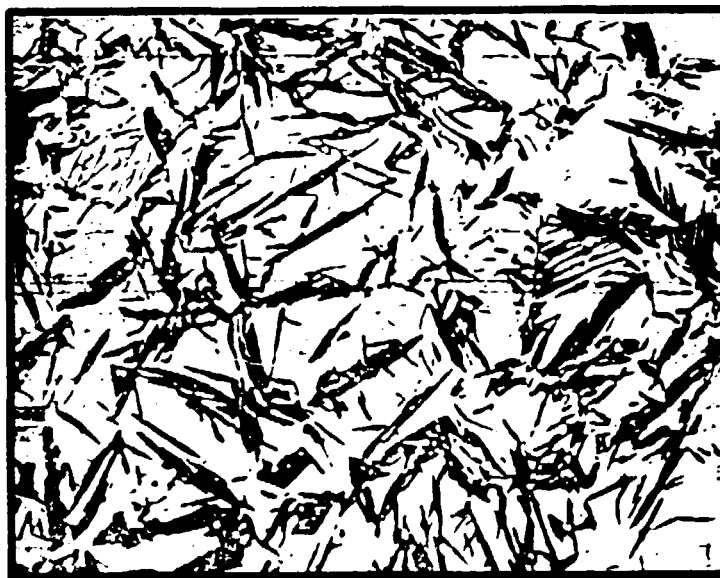
FIG 1.8 DARK NEEDLES OF MARTENSITE IN AUSTENITE MATRIX ( X 1000)
