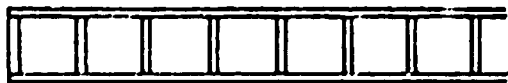
J. Simple truss beam with vertical webs (strength and stiffness is improved when webs are trenched in)
