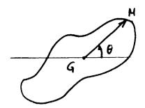
POLAR SIGNATURE Method consists in a tadially surreping of contour from the Gravity Center G of a given object <u>GM</u> = <u>GM</u>(θ) : "signature"
