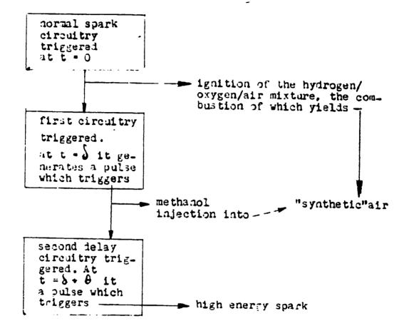
Since this procedure requires a more important equipment, in a first period of the trials one may simplify by using "real" air instead of "synthetic" air, loosing however the advantage of high temperature gases.
