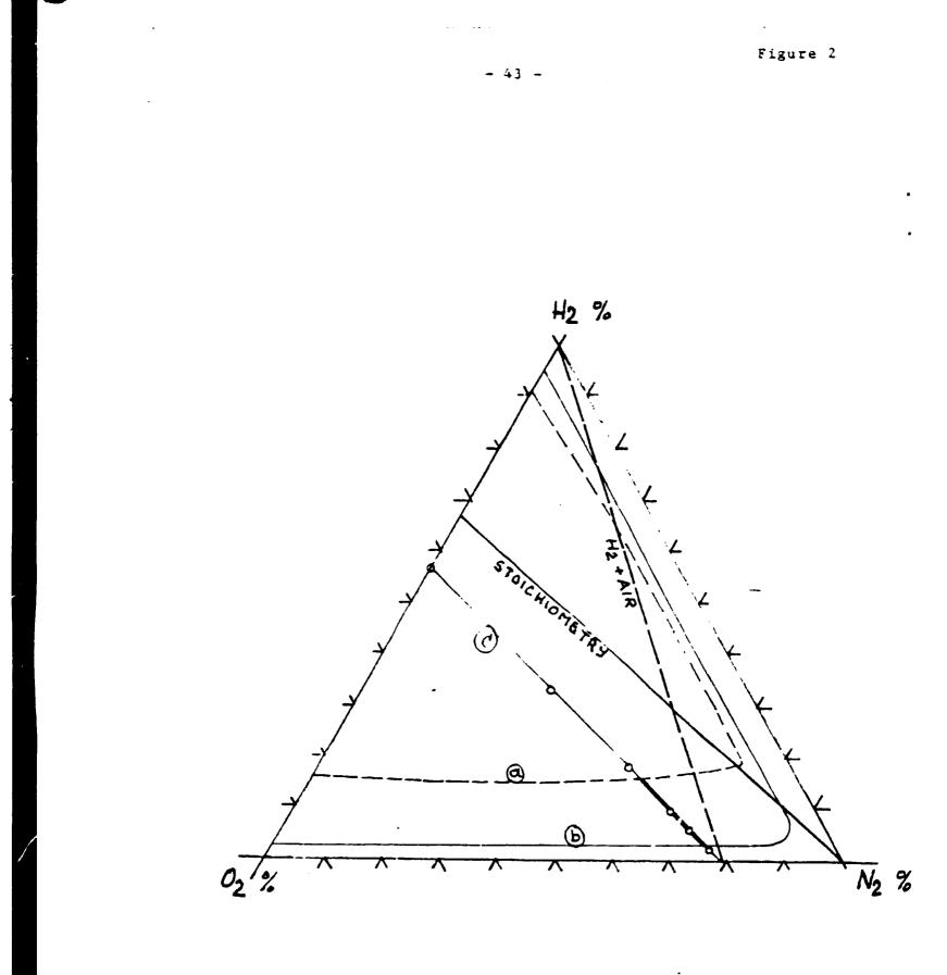
LIMITS(4) OF DETONABILITY -----(b) AND FLAMMABILITY -----AT NORMAL PRESSURE AND TEMPERATURE
