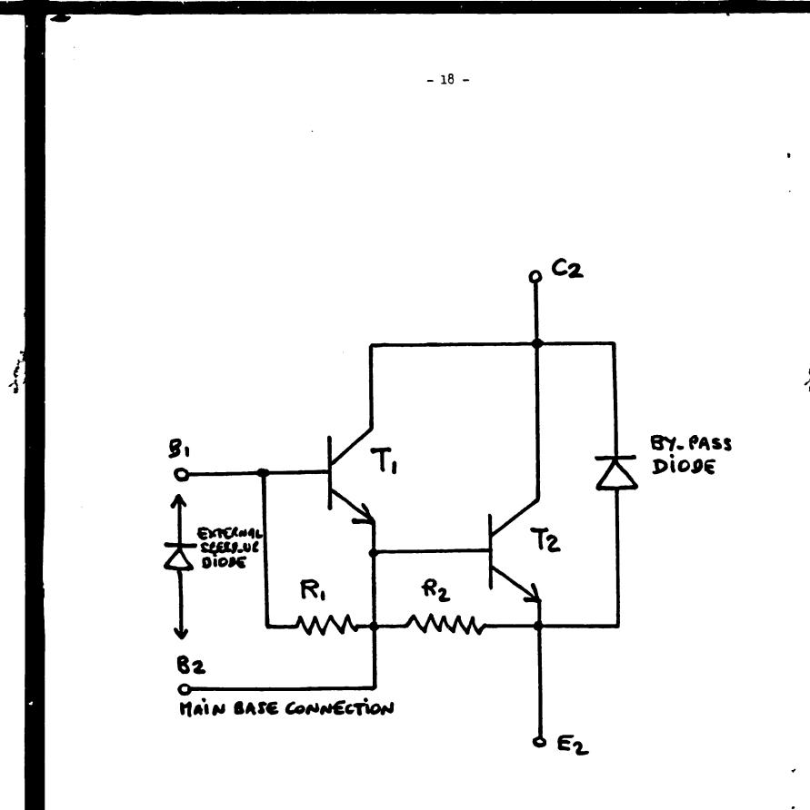
Fig. 4 - Additional main base connection.»
