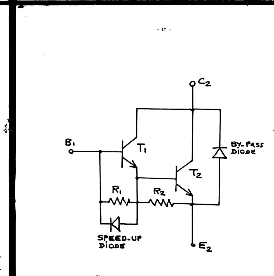
Fig. 3. - Speed-up Diode Connection.
