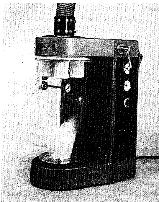
Figure 6.4 Aeromatic fluid-bed granulator, laboratory unit STREA-1 (by courtesy of Aeromatic AG; Bubendorf, Switzerland)
