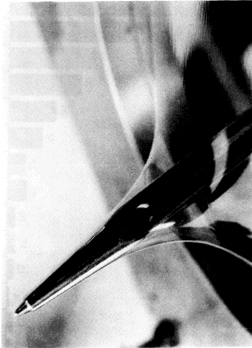
Figure 24. Puncture resistance test of Luflexen 0322 H
