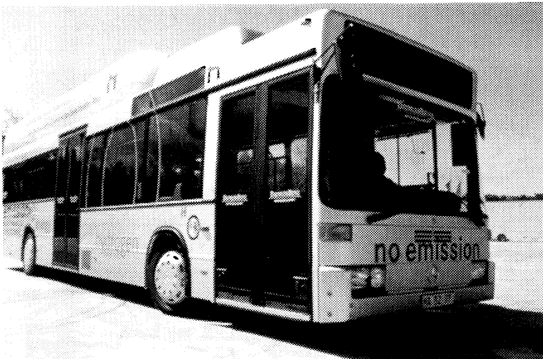
Figure 7.4: Daimler-Benz fuel cell bus (NEBUS) with compressed hydrogen storage
