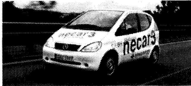
Figure 7.3: Daimler-Benz's fuel cell powered NECAR III prototype car
