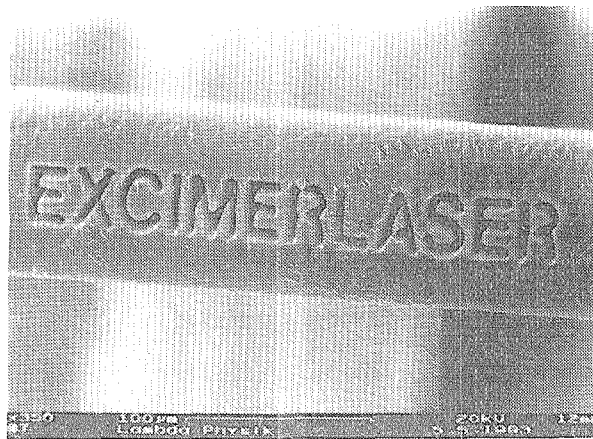
Figure 20 Human hair micromachined, with no discernible damage, by excimer laser mask projection (Courtesy of Exitech Ltd., UK)
