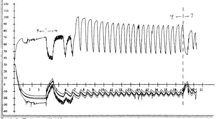
Mux. Temp. = -14.1°C > Thermostate position to 4
