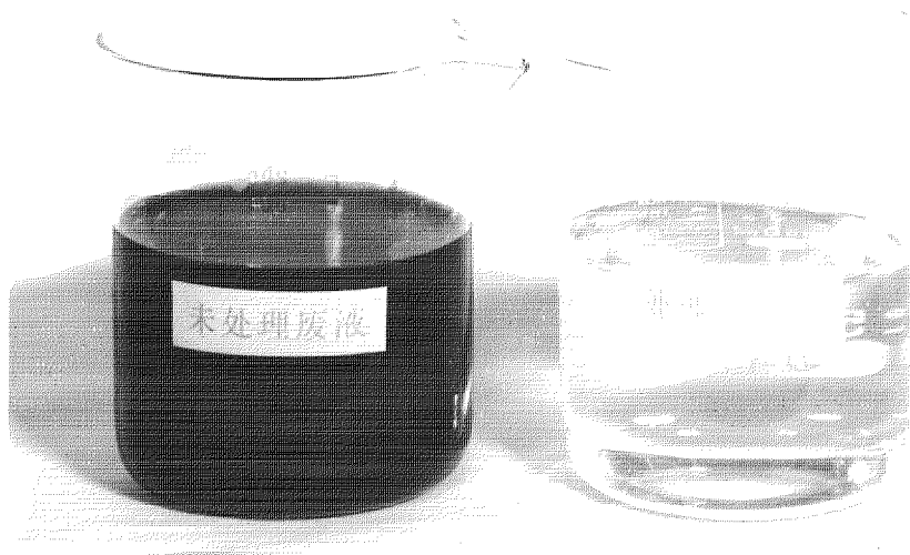
Figure 10: The treatment of waste water from mine explosives with DGB type decolourant
