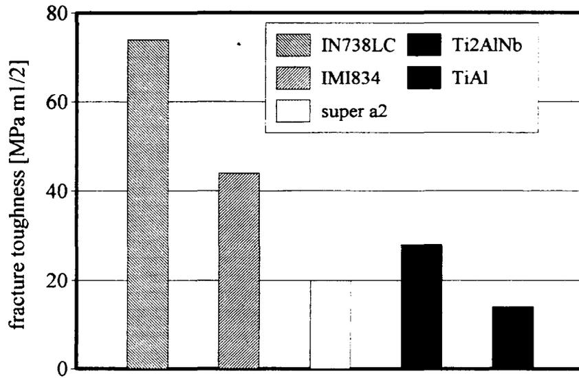
Figure 28: Room temperature fracture toughness  $K_{IC}$  of TiAl-alloys compared to Ni-base alloy IN738LC and Ti-alloy IMI834 [24]
