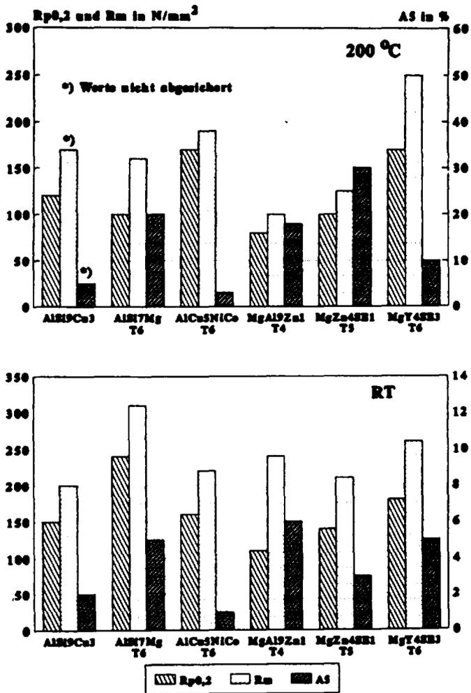
Figure 43: Properties of selected aluminium and magnesium alloys
