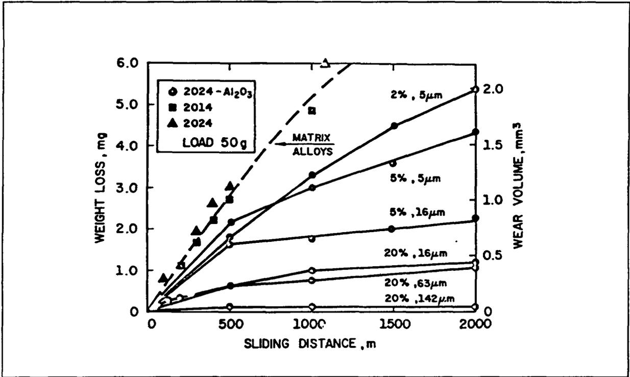
Figure 48: Weight loss vs. sliding distance for different particulate reinforced aluminium alloys
