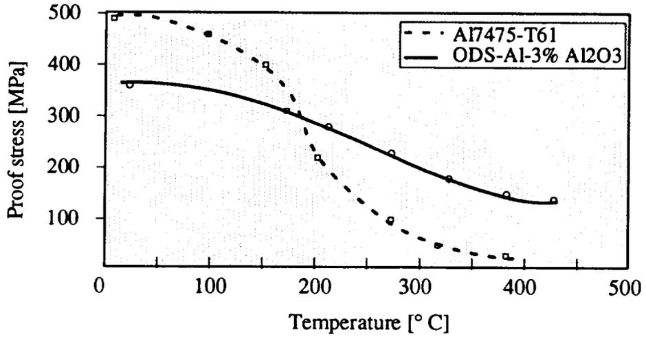
Figure 35: Proof stress of ODS-Al as a function of temperature, compared to Al7475 [Raufoss Inc., Norway]
