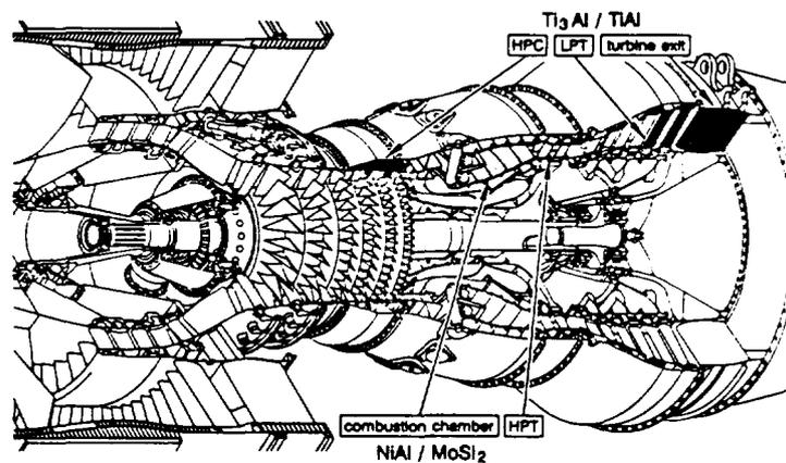
Figure 17: Application potential for intermetallic structural materials in gasturbines [24]
