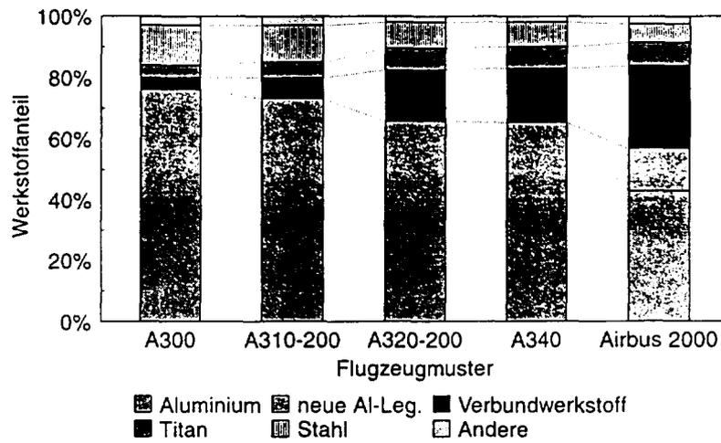
Figure 8: Content of different materials in aeroplanes
