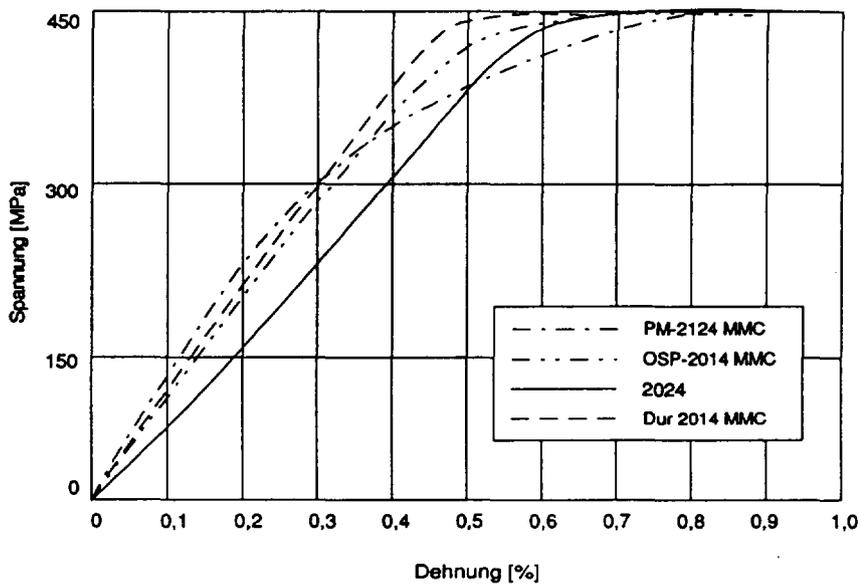
Figure 47: Comparison of the stress-strain behaviour of particulate reinforced aluminium alloys produced by different technologies. The 2024 alloy is not reinforced. PM means Powder Metallurgical, OSP means Spray Deposition (Osprey), Dur means Duralcan process (melt metallurgical)
