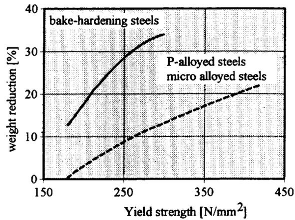
Figure 18: Weight reduction as a function of yield strength. Comparison between auto body structures (BH-steels) and crash elements (micro alloyed resp. P-alloyed steels) [32]
