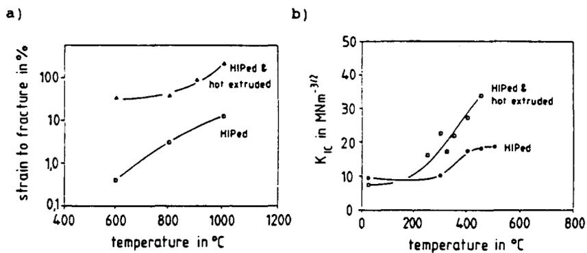
Figure 32: Temperature dependence of elongation and fracture toughness of NiAl-38.5Cr processed by HIP or HIP and extruding [36]
