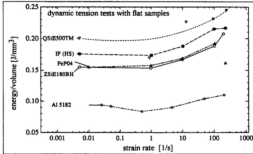
Figure 20: Dissipated specific energy of high strength steels during dynamic room temperature tests as a function of the strain rate [31]
