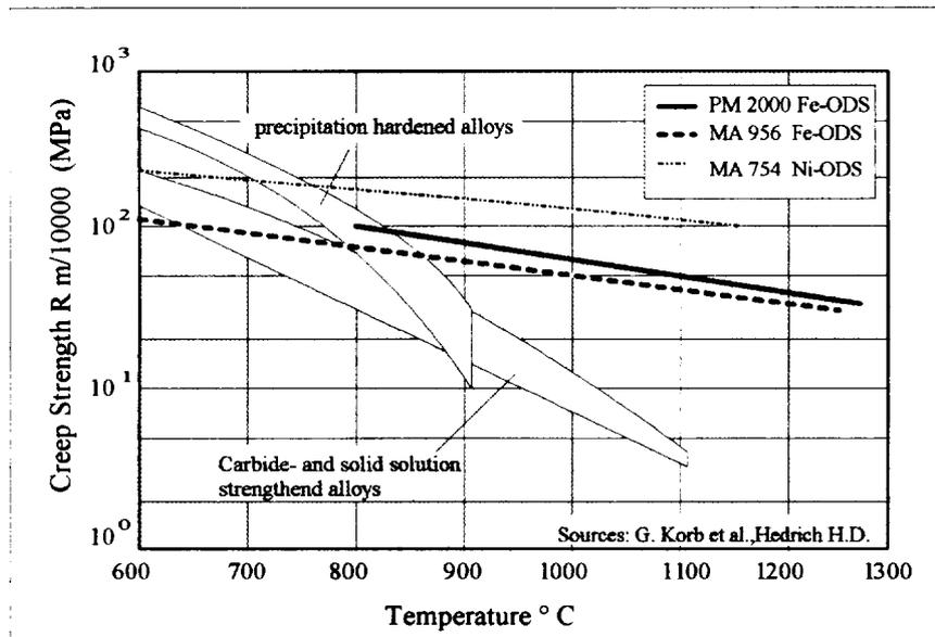
Figure 40: Creep behavior of ODS-Fe alloy PM2000 as a function of temperature, compared to standard high temperature alloys [54]
