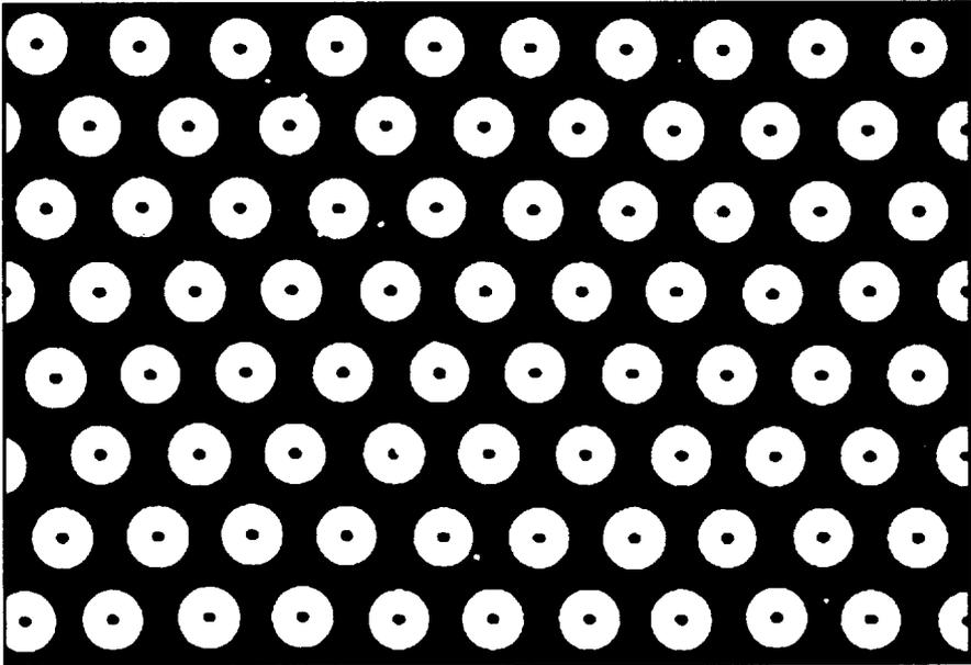
Figure 51: Cross-section of a SiC long-fibre reinforced titanium matrix composite
