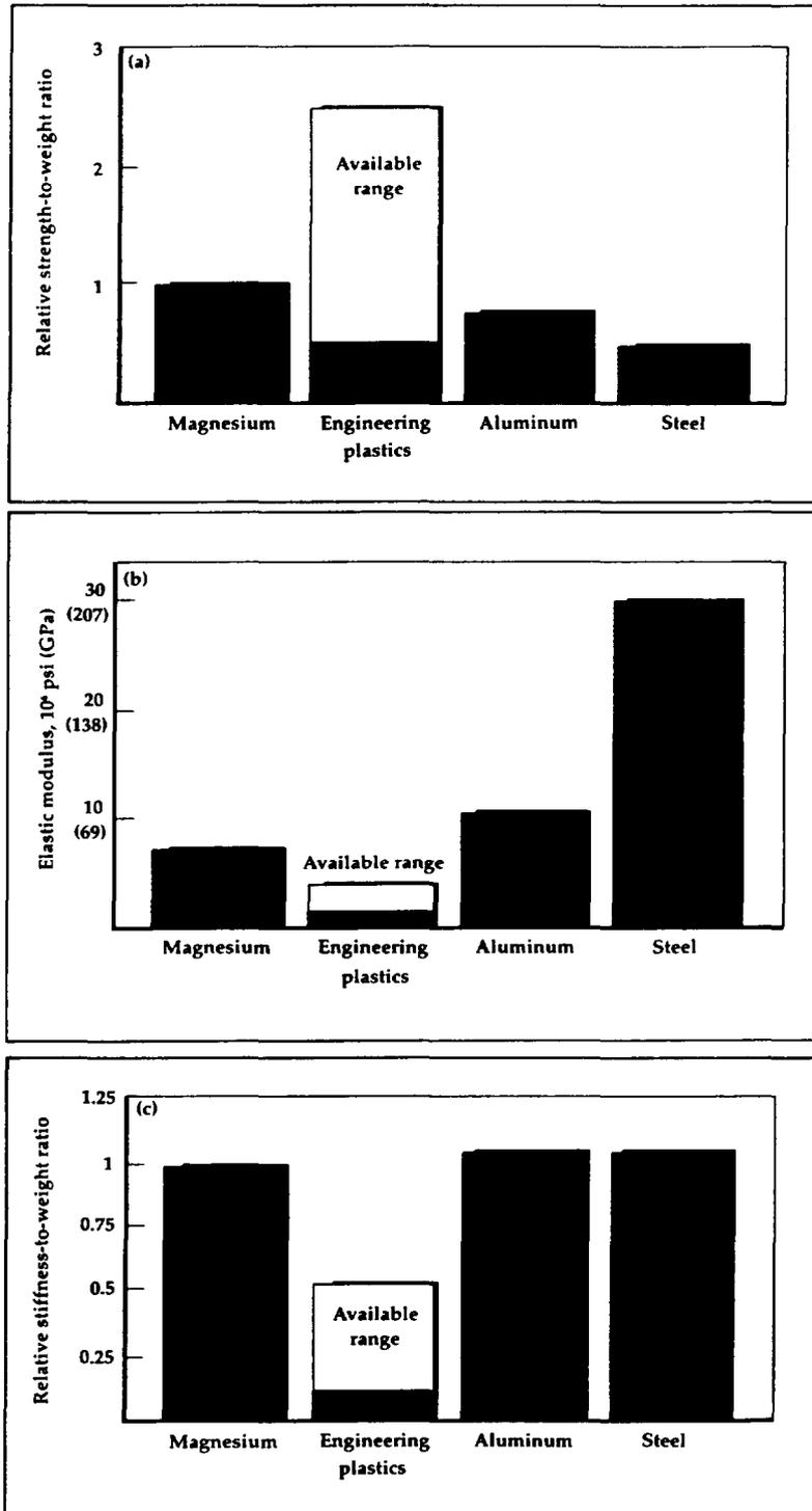
Figure 3: Property efficiency attributes of magnesium compared to those of selected other structural materials for auto applications. a) Relative strength-to-weight ratio. b) Elastic modulus. c) Relative stiffness-to-weight ratio.
