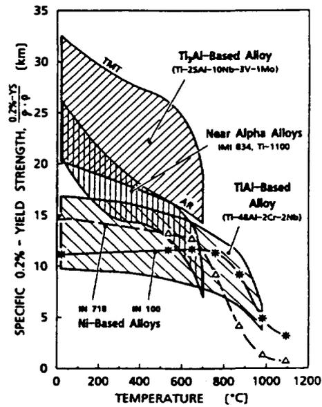
Figure 29: 0.2% yield strength of  $Ti_xAl$  as a function of temperature compared to conventional Ti- and Ni-base alloys [Kumpfert J. et al.]
