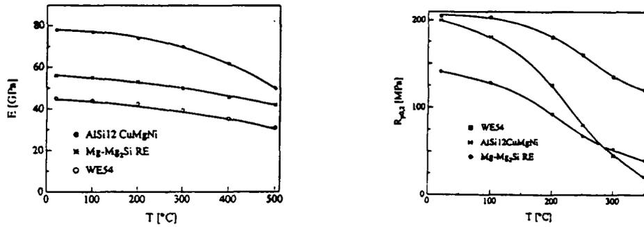
Figure 33: Youngs modulus and 0.2%-yield strength of Mg-Mg<sub>2</sub>Si as a function of temperature [44]
