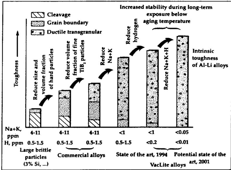
Figure 41: Increase of toughness as a function of the decrease of impurities for AlLi alloys
