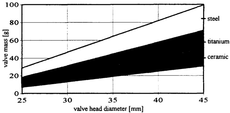
Figure 14: Masses of inlet valves [20]
