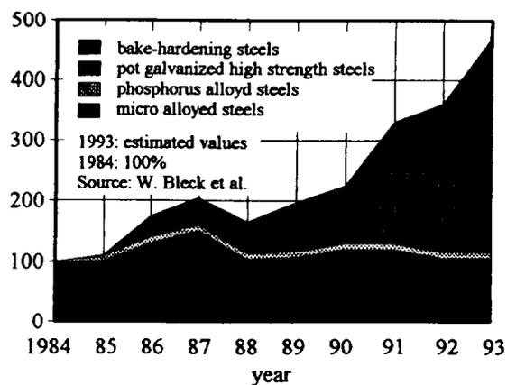
Figure 19: Increase in use of high strength steel strips in automotive industry [30]
