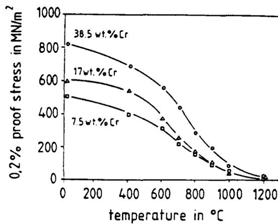
Figure 31: 0.2% proof stress of NiAlCr as a function of temperature and Cr-content [36]
