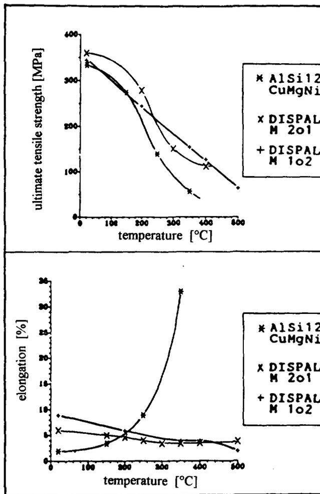
Figure 38: Ultimate tensile strength and elongation of different dispersion strengthened Al-alloys as a function of temperature [50]
