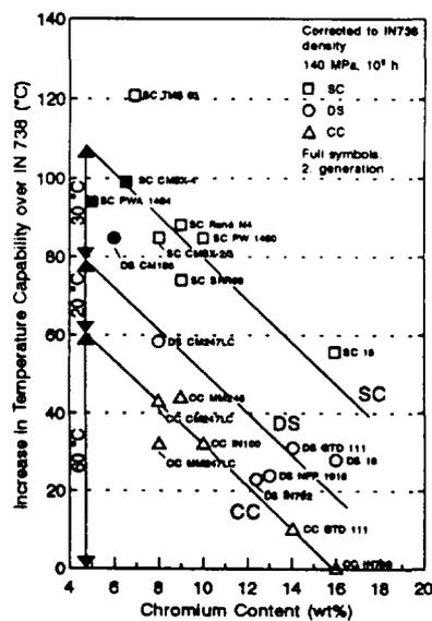
Figure 27: Maximum operation temperature of Ni-base alloys as a function of Cr-content. The temperatures are defined by creep resistance. The values are related to the creep strength of Ni-base alloy 738 [23/33]
