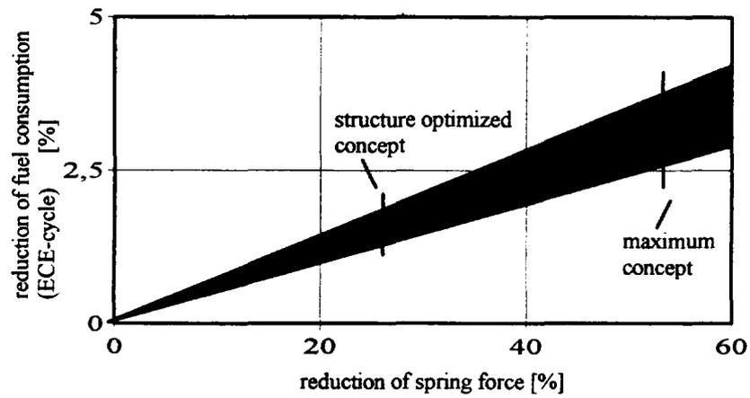
Figure 13: Reduction of fuel consumption with decreasing valve spring force (ECE-cycle) [20]
