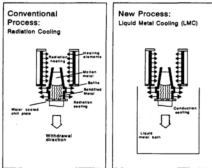
Figure 26: Comparison of conventional cooling and liquid metal cooling during directional and single crystal solidification [23]
