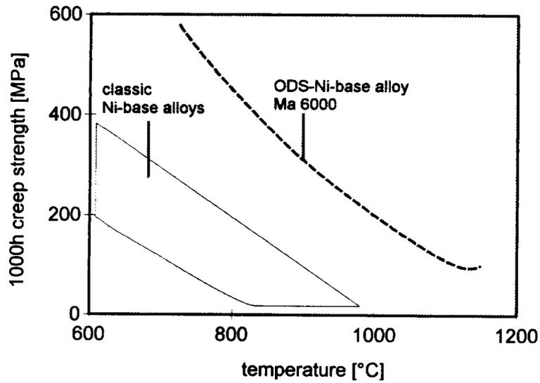
Figure 39: Creep behavior of ODS-Ni-base alloy MA6000 as a function of temperature, compared to standard Ni-base alloys
