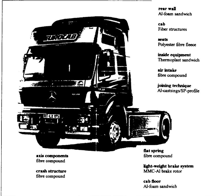
Figure 4: Light-weight construction concepts for a lorry
