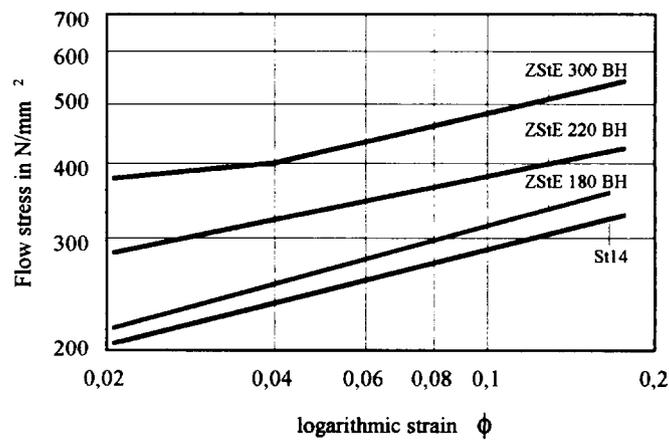
Figure 21: Flow stress of bake-hardening steels compared to steel St14 [30]
