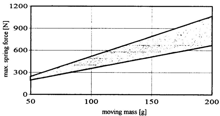
Figure 12: Required spring force of serial motors (related to the nominal rate of revolutions 6250 1/min) [20]
