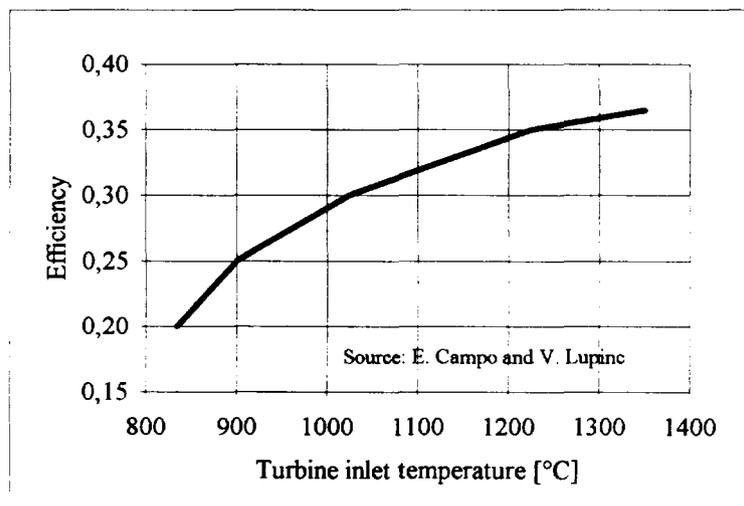
Figure 15: Increase in thermal efficiency with increasing gas temperature at turbine inlet [24]
