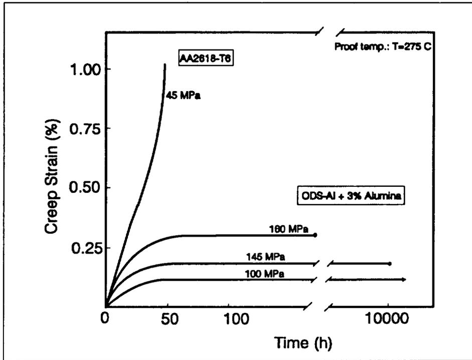
Figure 36: Creep behavior of ODS-Al (Al + 3% alumina) [Raufoss Inc., Norway]
