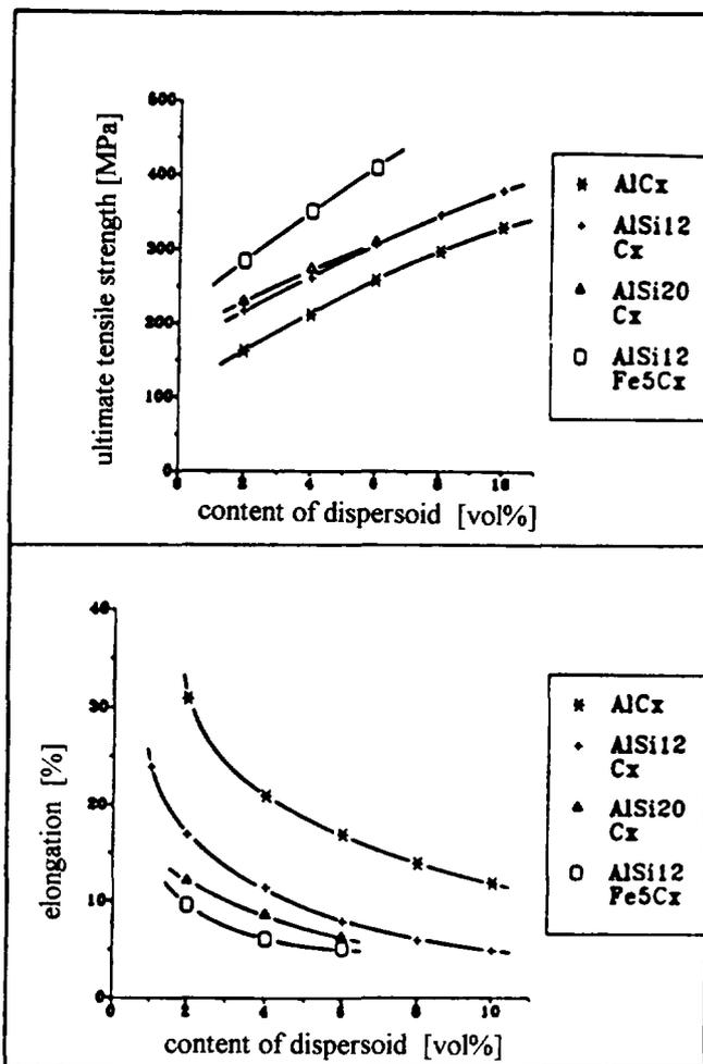
Figure 37: Ultimate tensile strength and elongation of different dispersion strengthend Al-alloys as a function of dispersoid content [50]
