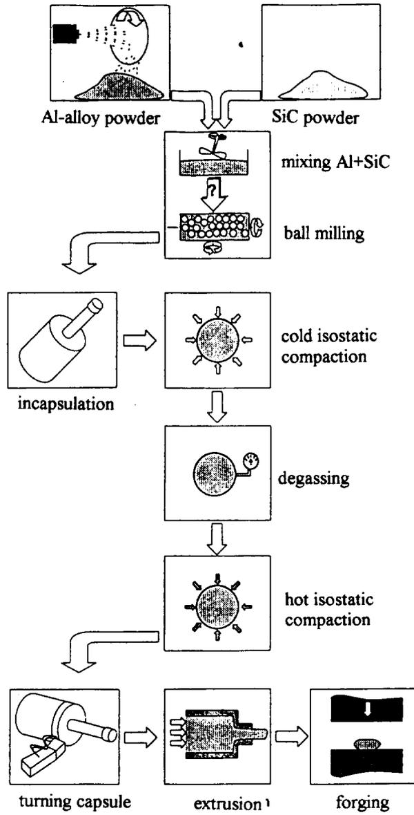
Figure 45: Powder-metallurgical production of particulate reinforced aluminium
