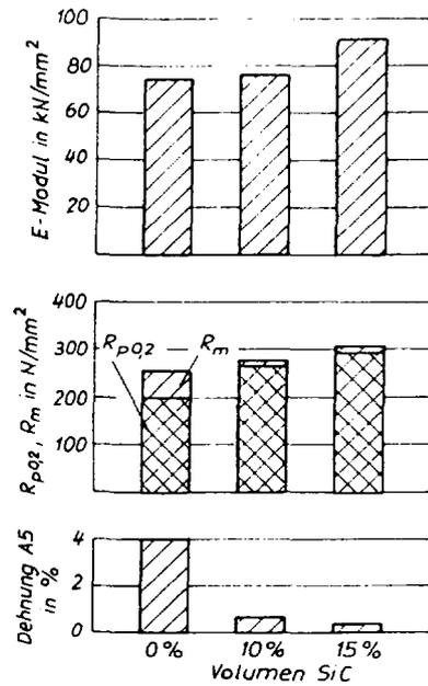
Figure 46: Typical properties of melt metallurgical produced particulate reinforced aluminium
