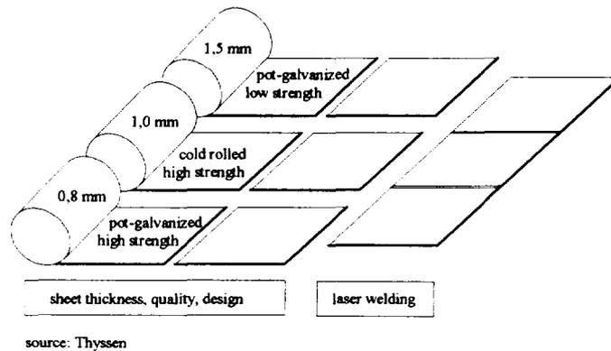
Figure 23: Schematic description of the production of tailored blanks [32]
