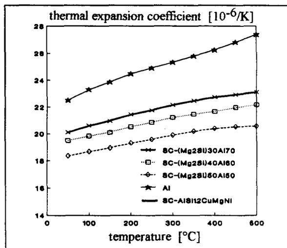
Figure 34: Coefficient of thermal expansion of different Mg-Mg<sub>2</sub>Si alloys as a function of temperature, compared to standard piston alloy [18]
