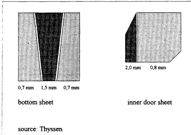
Figure 24: Examples of the design of tailored blanks [32]
