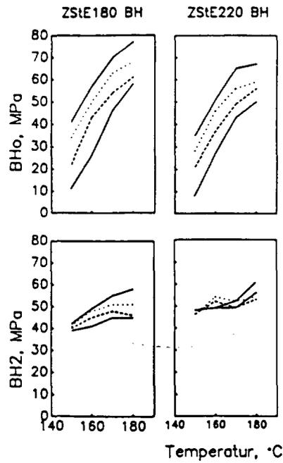
Figure 22: Influence of temperature and time on the bake hardening effect BH0 (without pre-deformation) and BH2 (2% pre-deformation) [29]
