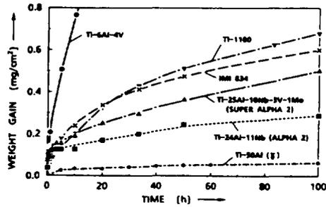
Figure 30: Oxidation behavior of titanium alloys [37]
