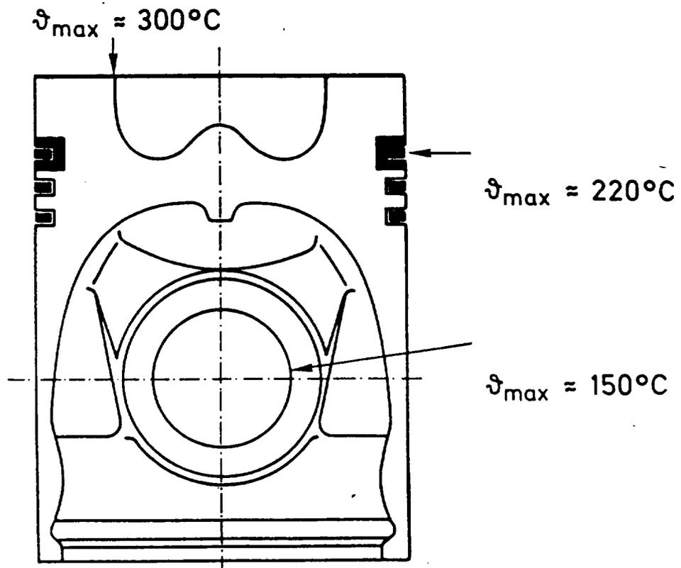
Figure 11: Critical piston sections [17]
