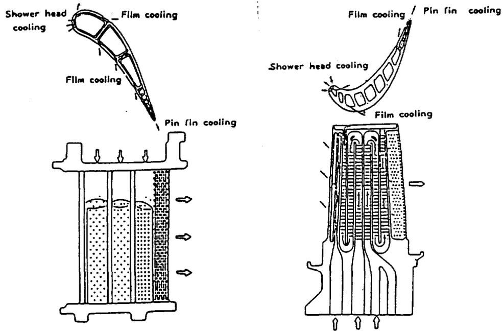
Figure 16: FMW 701F first stage airfoils geometry: a) nozzle guide vane and b) blade [24]
