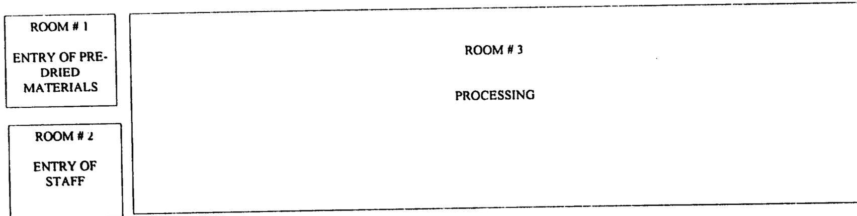
*Note that owing to the cost of maintaining the humidity / temperature conditions required for handling effervescent products it is acceptable practice to minimise production areas and segregate processing areas within a single room.*
