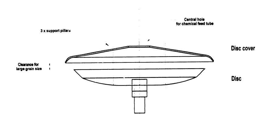
Figure 2 : Cover arrangement for the liquid spreading disc to minimise contact of seed with the disc surface
