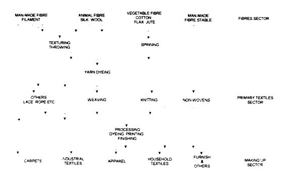
Figure 1: Structure and Material Flow of the Textiles Industry
