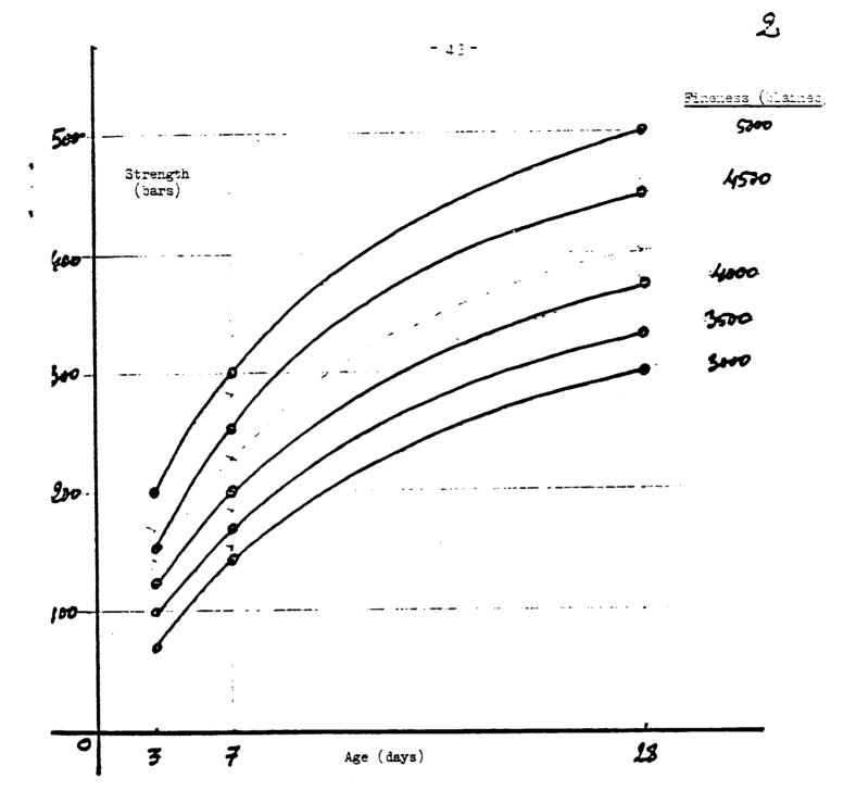
Compressive strength of mortars made from cement (3000 blaines) with 75% slag of varying fineness (cement and slag ground separately)
