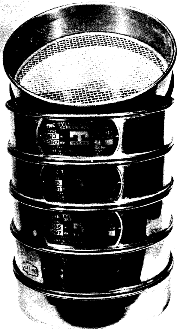
Figure 2. Set of Test Sieves as Used for Determination of Particle-Size Distribution in Fertilizer.
