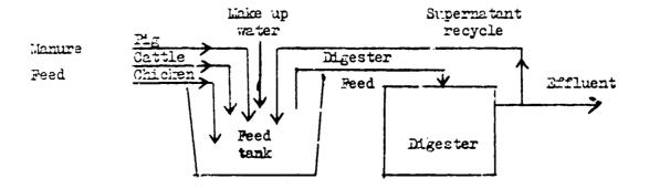
Normally results of digester operation are expressed in terms of the relationship between feed and effluent stream properties such as total solids %, volatile solids % etc. and these are derived from mass balances based upon this flow sheet.
