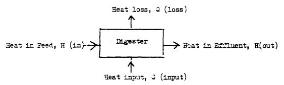
In a steady state, the heat required to maintain the digester at its desired temperature, is given by the expression below (Units Reals/day)
