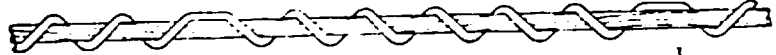
Fig. 2: Diagram showing the structure of the combined synthetic filament and staple wool yarn produced by the Selfil machine. The upper illustration shows the yarn with a single binding filament as produced by the first twisting stage, while below is the completed yarn after leaving the second twisting stage; this yarn, of course, has two filament binders.
